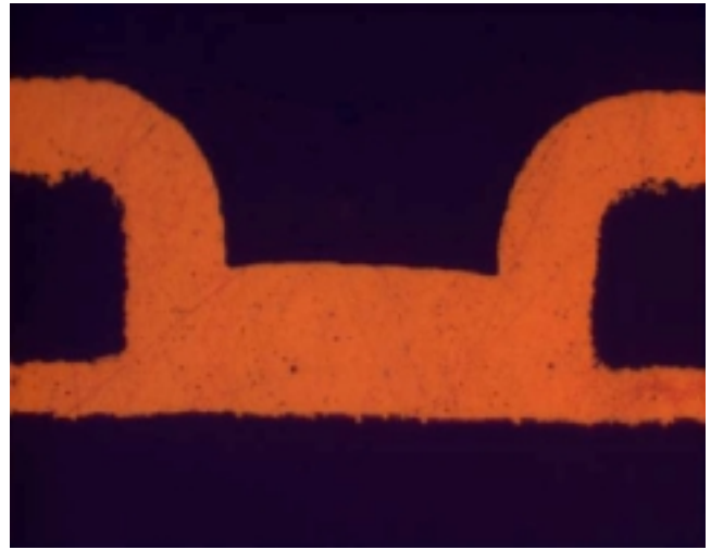
b. Cross Section of a Photo Processed Via from Vendor 4
