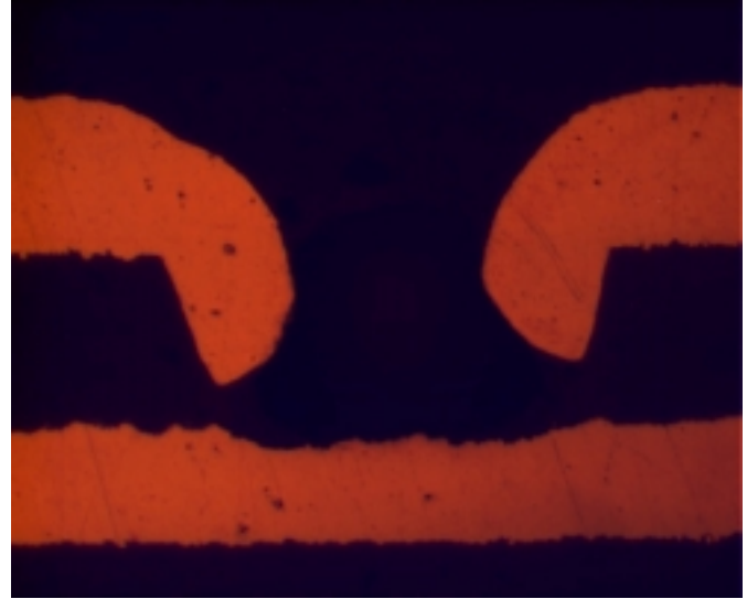
b. Cross Section of an Improperly Plated YAG Laser Drilled Via from Vendor 2 (Time Zero Cross Section)
