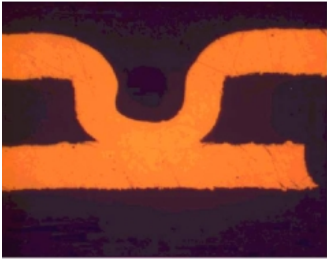
a. Cross Section of a YAG Laser Drilled Microvia from Vendor 1
