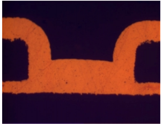
b. Functional Via after 2000 LLTS Cycles
