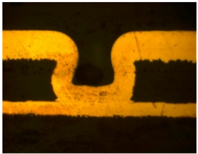
b. Cross Section of a Photo Processed Via from Vendor 4
