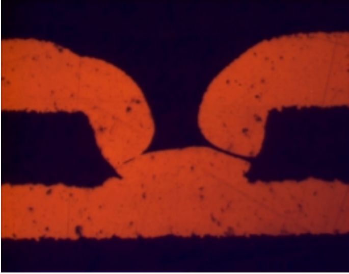
a. Cross Section of a Via with a Break in the Hole Wall (Time Zero Cross Section)
